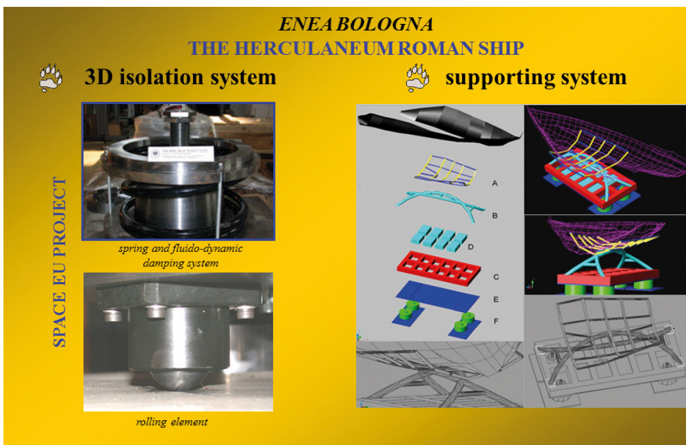
Figure 14: The Herculaneum Roman boat: 3D isolation and supporting systems.
