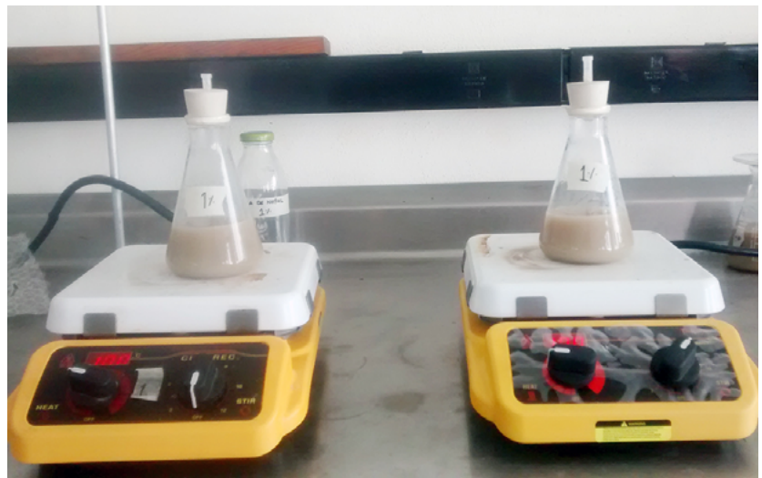
FIGURE 4. Hydration process of Opuntia ficus indica nopal gum powder (Picture: Josué Israel Moreno Fraga, 2020).
