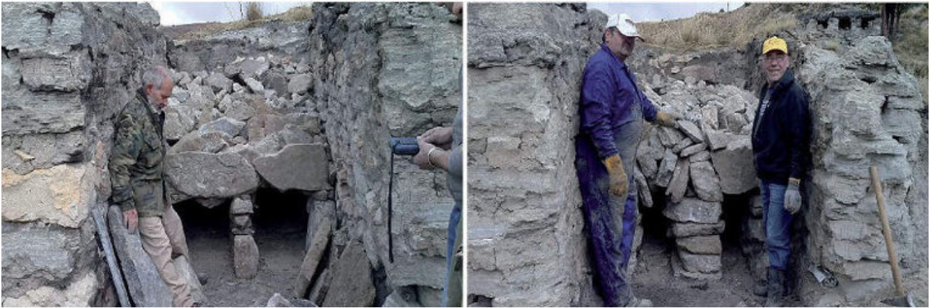
Figure 4.- Old masons placing gypsum stones in the oven, Navarrete.
