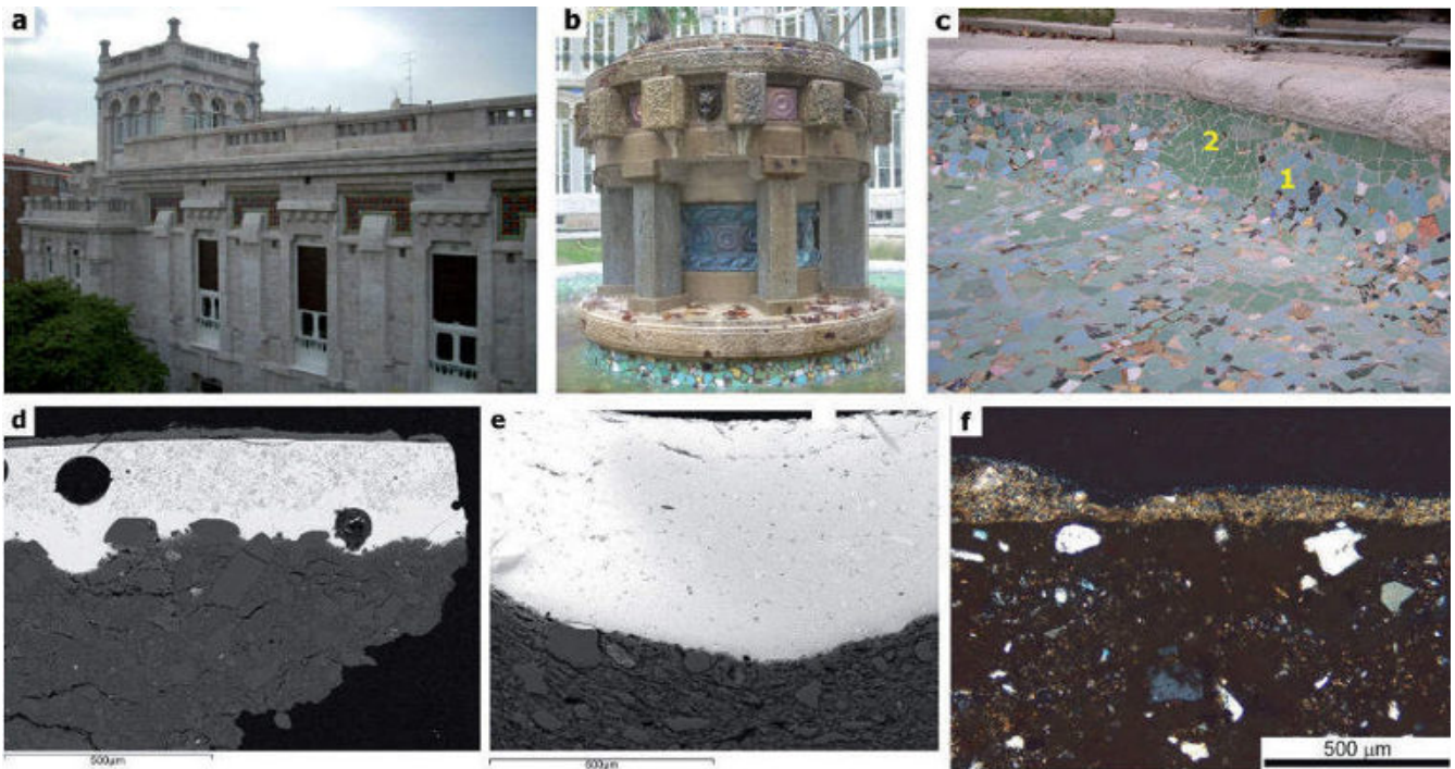
Figure 3.- Decorative ceramics: ceramic panels and tile trencadix . a: upper part of façades decorated with ceramic panels; b: original raindrop tiles on the body of the central fountain; c: basin of the fountain adorned with tile trencadix -original tiles (1) and tiles placed at 80s (2)-; d: original tiles manufactured by Zuloaga and e: tiles elaborated at 80s (both SEM-BSE mode images) -differences on texture and on ceramic body/glazes contact were observed-; f: polarised optical micrograph of the original tile trencadix (crossed nicols), quartz inclusions in ceramic body and the glaze applied on the ceramic body were observed.
