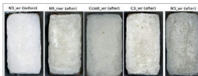
Figure 1. - Scans of some of the specimens before (b) and after (a) the crystallization cycles.
