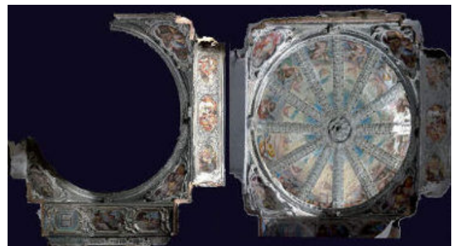
Figure 1.- Orthophotograph made from the three-dimensional model of the dome of the Purification Chapel of the church of Santa Maria del Carmine in Milan, Italy.
